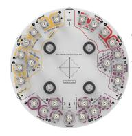
24-port small cell antenna, 4x 617-960, 8x 1695-2690, 8x 3400-4000 MHz beamformer, 4x 3100-4200 MHz, 360° Horizontal Beamwidth, fixed tilt.
