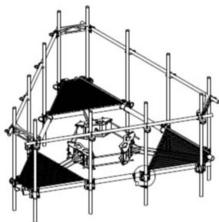
3-Sector Monopole Co-location Platform Kit, 10 in to 30 in OD, 12 ft 6 in face, includes twelve 96 in pipes
