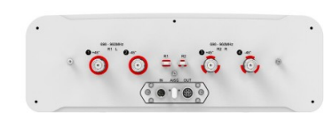
4-port sector antenna, 4x 698–960 MHz, 65° HPBW, 2x RET
