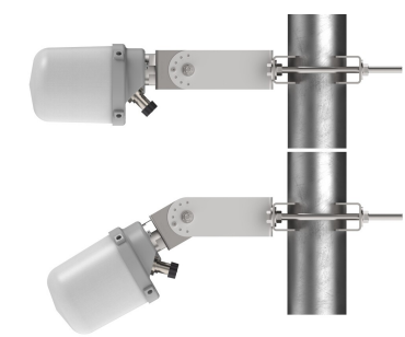
2-port Venue Antenna, 3300-4000 MHz, 37° HPBW, Fixed Tilt
