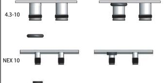
2 Loosen nut 2 from sleeve by approximately 5 mm (as shown in Figure 1), or fully detach it from sleeve (as shown in Figure 2). Then, push sleeve forward to cover the gasket, ensuring it is aligned with the gasket and stops against the face of the end cap (as shown in Figure 3). If nut 2 does not move together with sleeve manually screw nut 2 onto sleeve (as shown in Figure 4).
